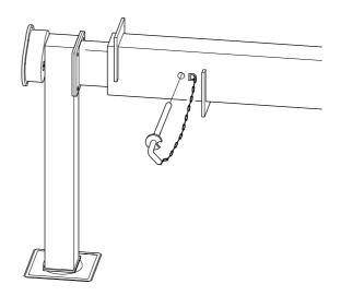
Fig.8-6 Locking pin outrigger
