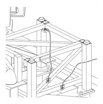
Fig.6-47 Lightning protection
