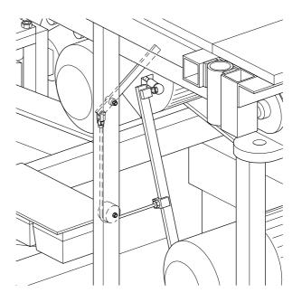
Fig.8-1 Drive unit brake release
