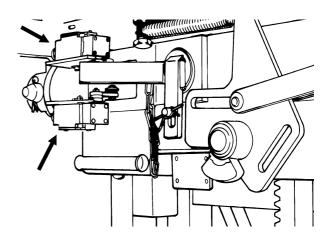
Fig.6-45 Autolevel switches
