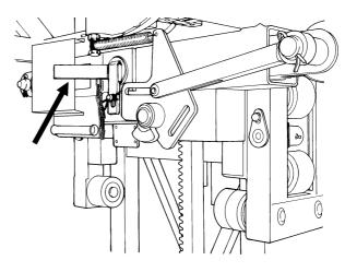
Fig.6-17 Autolevel locking pin
