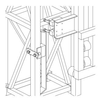
Fig.6-43 Adjusting lower striker plate
