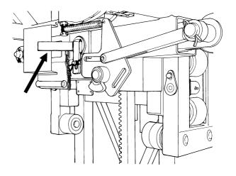
Fig.6-24 Autolevel locking pin
