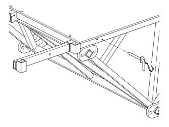
Fig.8-4 Securing outrigger
