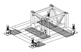
Fig.6-3 Ground support ground frame
