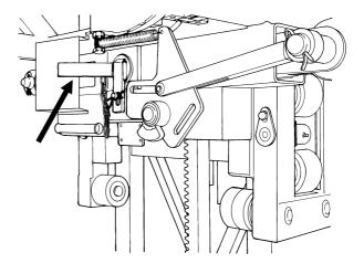
Fig.6-22 Autolevel locking pin
