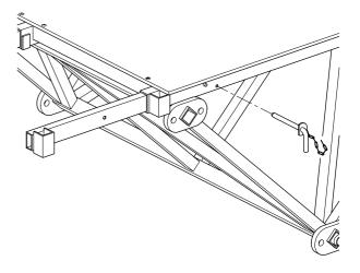
Fig.6-38 Outrigger platform extension
