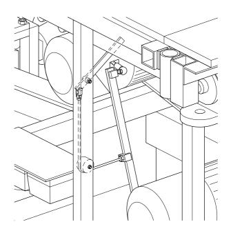
Fig.6-44 Brake lever drive unit
