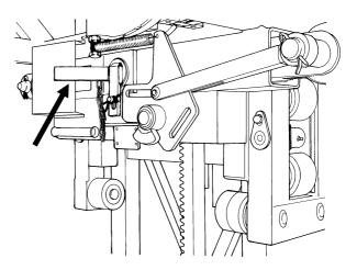
Fig.6-13 Autolevel locking pin
