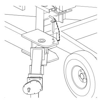
Fig.4-2 Locking pin outrigger chassis
