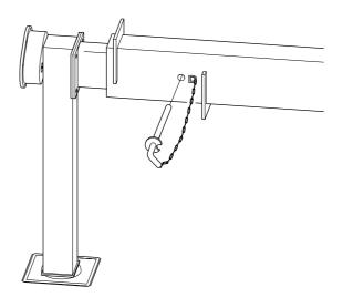
Fig.6-5 Locking pin outrigger chassis
