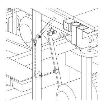
Fig.7-3 Brake lever drive unit
