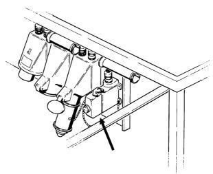
Fig.6-23 Control cable dummy plug
