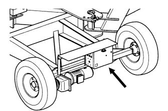
Fig.5-2 Power supply socket chassis
