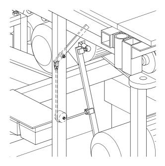
Fig.7-5 Drive unit brake release
