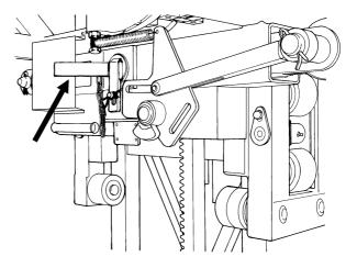
Fig.8-2 Autolevel locking locking pin
