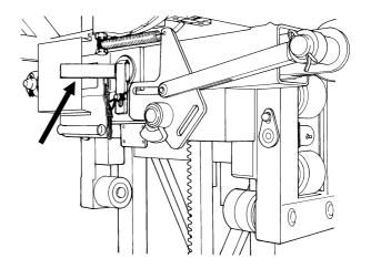
Fig.6-6 Autolevel locking pin
