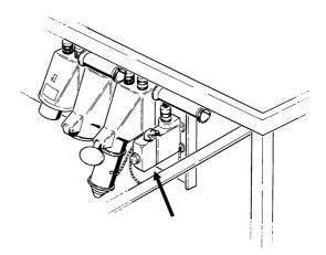
Fig.8-3 Control cable dummy plug
