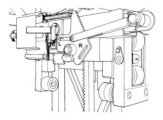
Fig.6-40 Machine setting left
